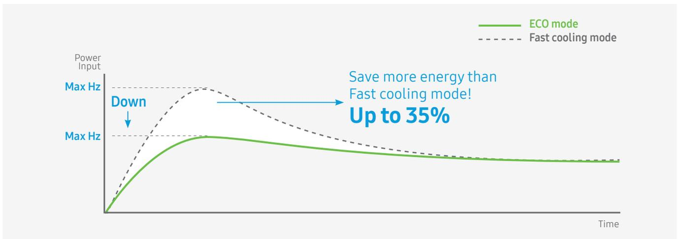
ECO mode operates at lower compressor capacity comparing to Fast Cooling mode, suitable for the mild days when it's not too hot. It minimises energy consumption, while still maintaining a cool and comfortable space.<sup>9</sup>
